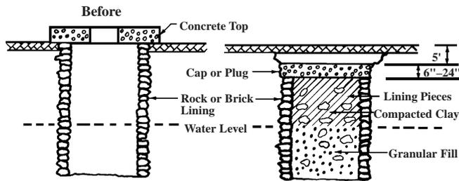
where centrifugal or shallow well jet pumps can be used. Driven or sandpoint wells are still being installed. To be legal, however, they must be grouted to a depth of 20 feet or to the water table. Because of shallow depths and grouting difficulties, they are discouraged for domestic use.
